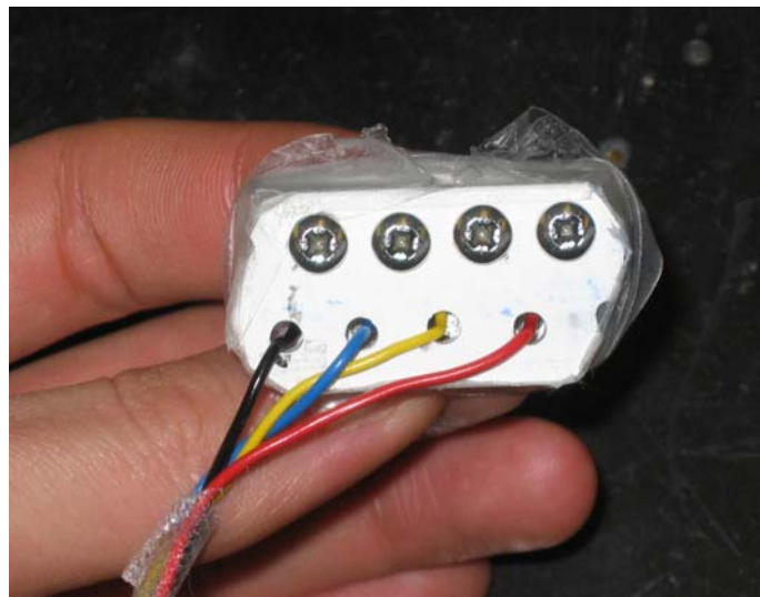
Figure 4.5 - Electrode probe used for measurement of local impedance changes.
